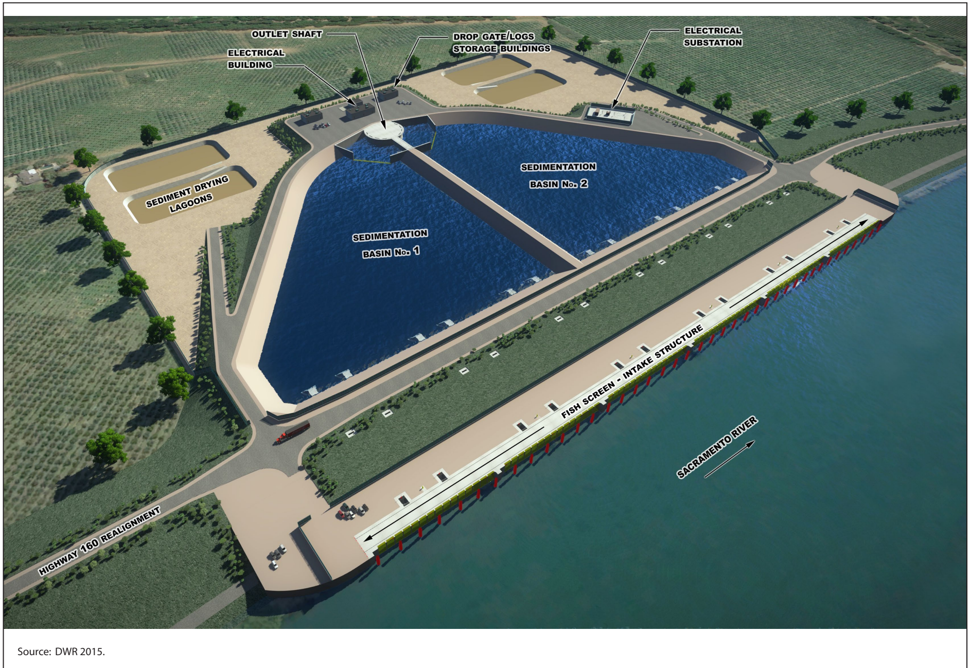
Figure 3-19a Conceptual Rendering of On-Bank Intake Facility for Alternative 4
